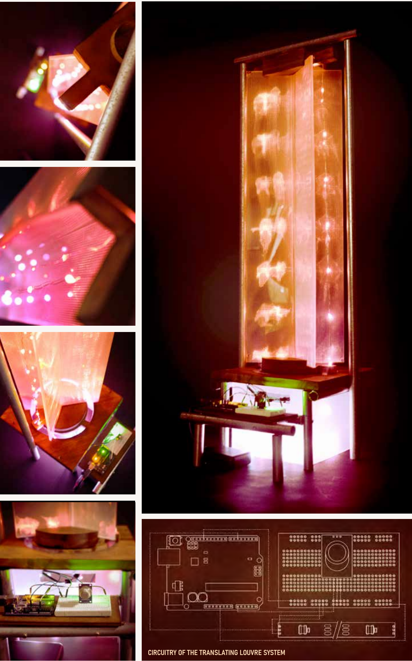
1:3 PROTOTYPING OF THE TRANSLATING LOUVRE SYSTEM
