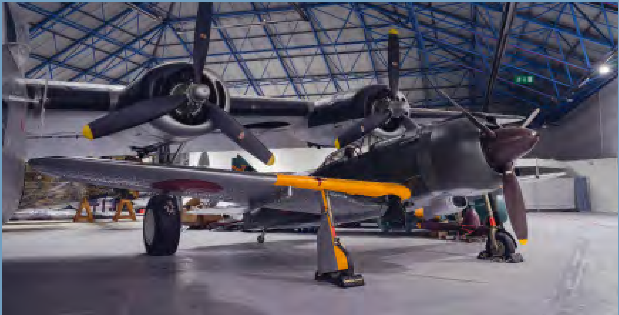
The Ki-100 is an emergency development of the liquid-cooled inline-V12 piston engined Ki-61 Hien (Swallow Tail), which had the original piston Ha40 engine replaced by a Ha112 14-cylinder radial engine, the resulting aircraft greatly resemble the infamous Mitsubishi A6M Zero fighter operated by the Imperial Japanese Navy Air Service
