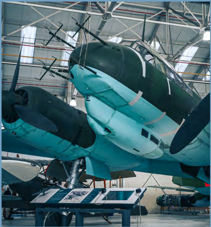
The Ju-88 utilize a pair of BMW 801 14-cylinder radial engines, in which the BMW logo can be seen on the engine cowling.
