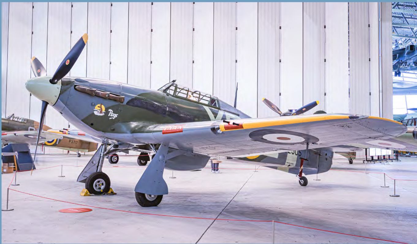
BE505, not just the only twin-seater Hurricane in the world, it is also the only flying “Hurri-bomber” Hurricane Mk.IIB variant, that being said, Hurricane Heritage have removed the underwing bomb rack from the aircraft.
