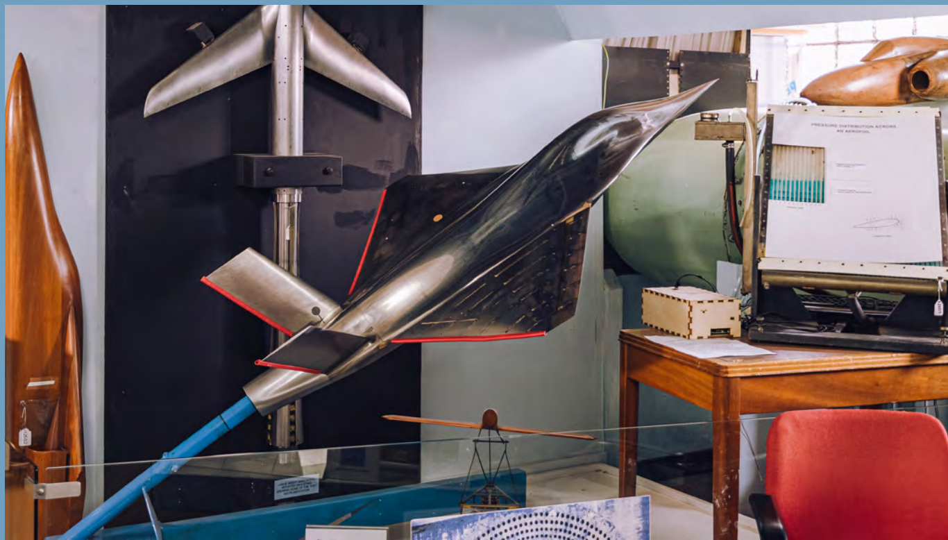
FAST's extensive collection of wind tunnel models includes this stealth model, the last designed by the RAE Bedford site, developed for the Future Air Offensive System (FOAS) program which was cancelled when the MoD opted for the United State's F-35 Joint Strike Fighter Program.
