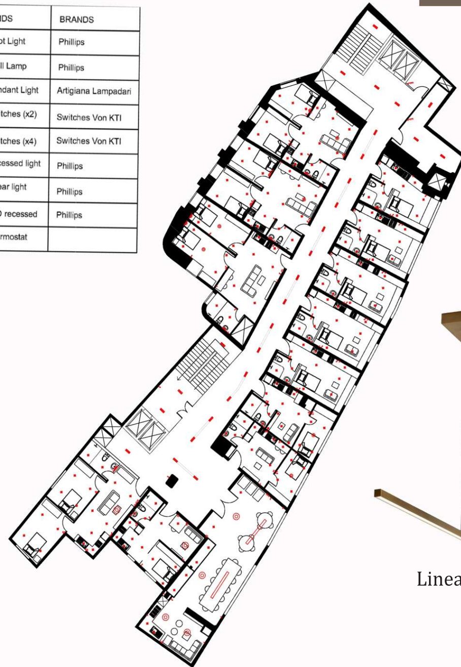
Second floor Electrical Plan
