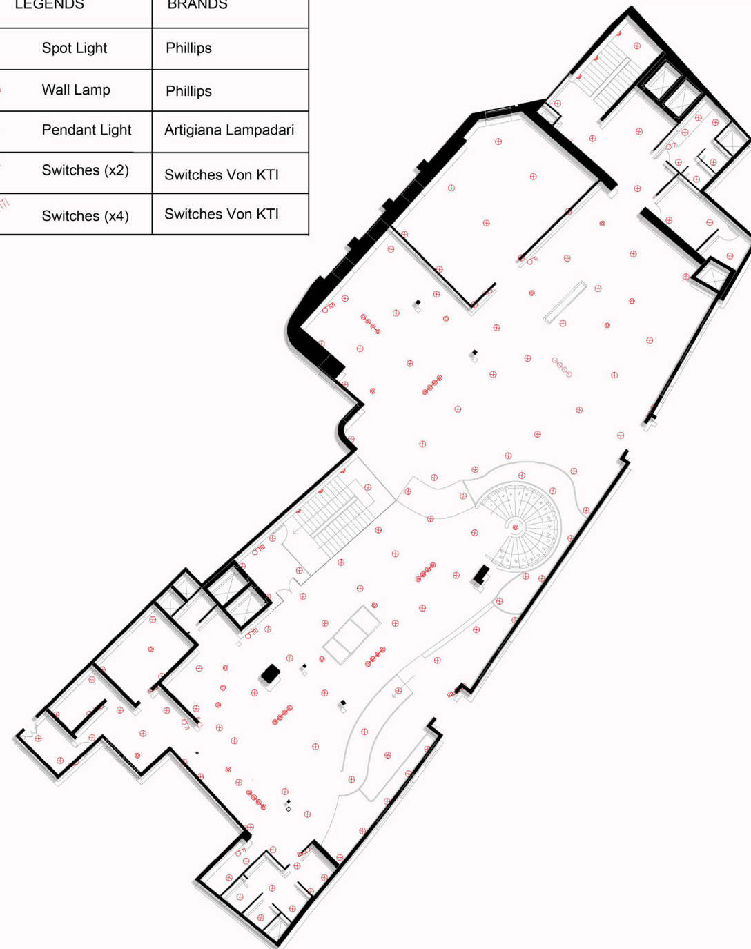
Ground Floor Electrical Plan
