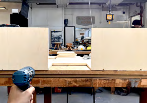
WOODEN FRAME plywood glued and screwed to place
