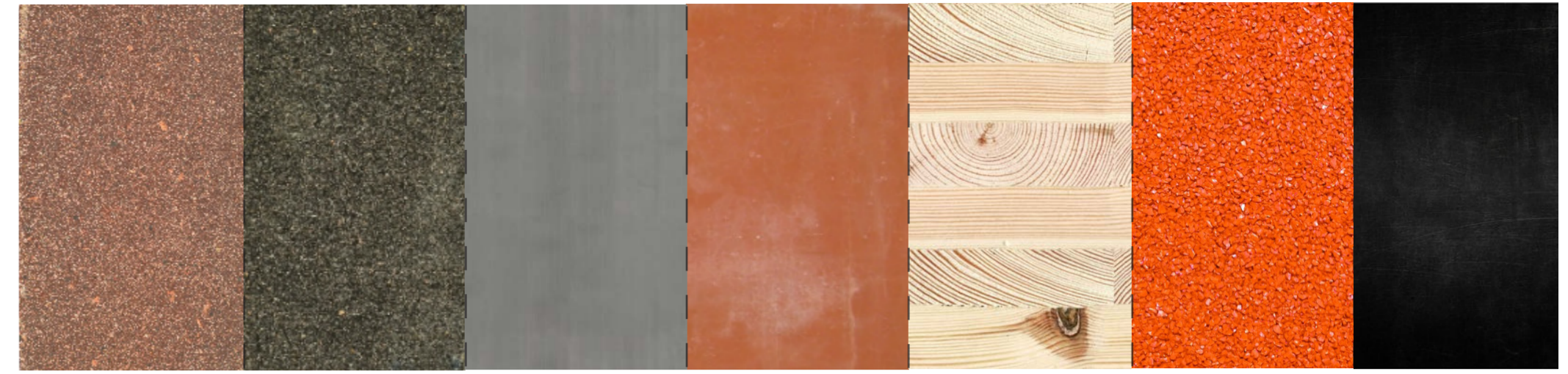
Burnt Orange K-BRIQ | Grey K-BRIQ | Brushed Aluminium | Red Viroc Panel | CLT Structure | Playground Rubber | Structural Steel
