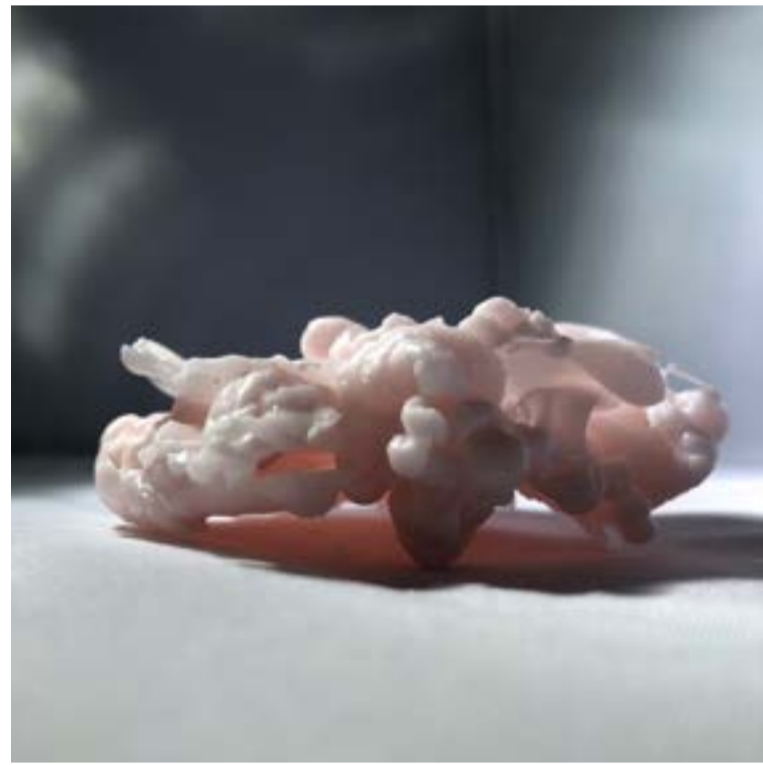
Wax experimentation by pouring hot wax in cold water
