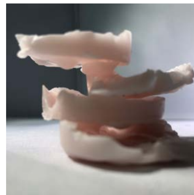
Wax experimentation by pouring hot wax in cold water
