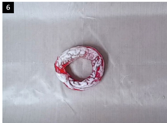
6. Create a circle out of the elongated tube by securing the edges. At this stage, the HDPE has solidified. It will help to melt it again to make it softer for further molding.
