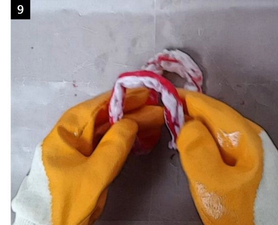
9. Shape the plastic by hands, creating a sideways 'U' shape. Hold the plastic in the 'U' shape till it solidifies.
