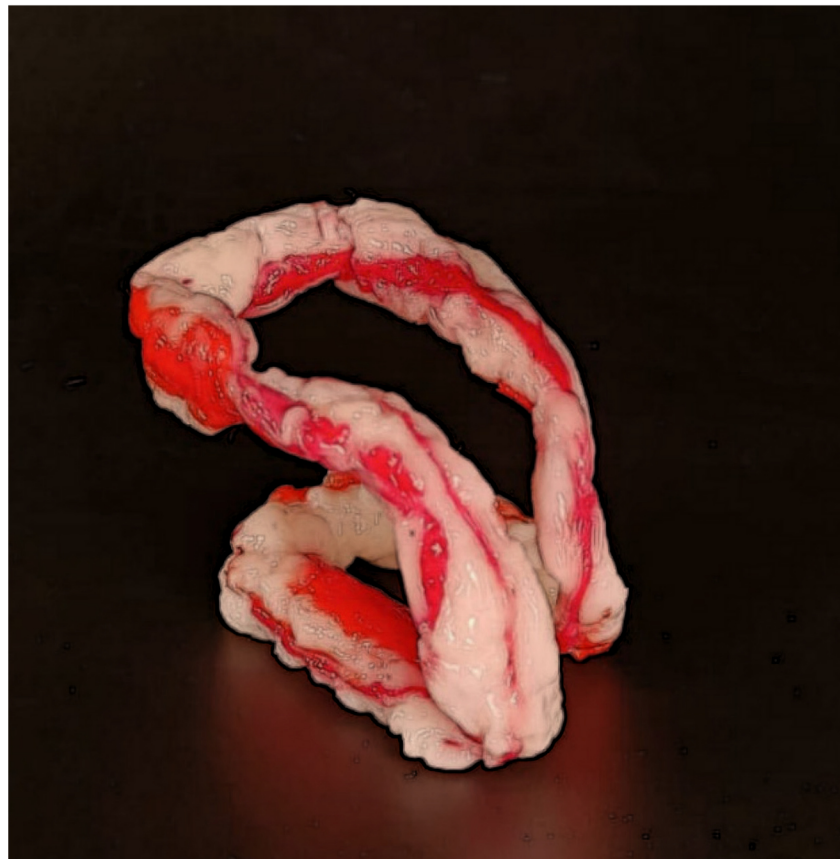
6. Create a circle out of the elongated tube by securing the edges. At this stage, the HDPE has solidified. It will help to melt it again to make it softer for further molding.
