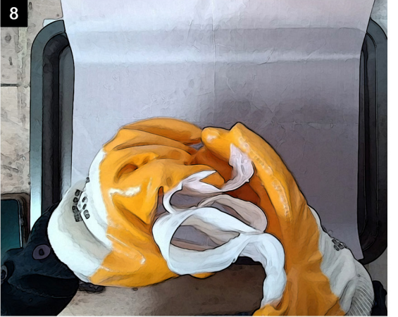
8 Hold the plastic in the wave pattern till it solidifies. Solidified HDPE turns into opaque white from transparent.
