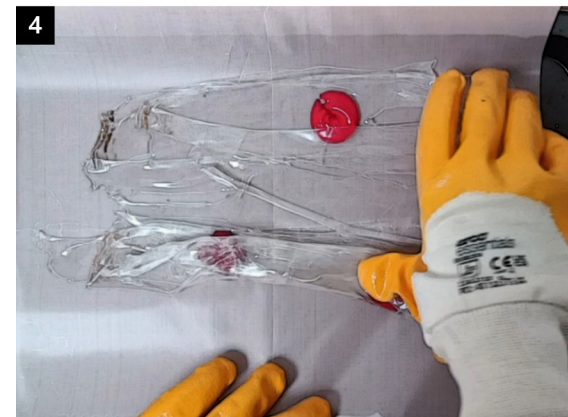
4. Roll the HDPE onto itself, removing it from the cooking liner.
