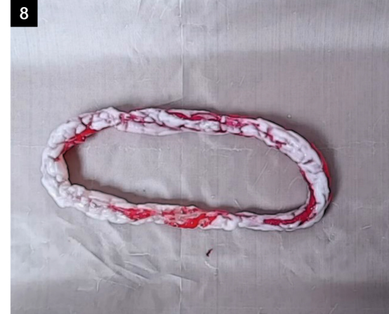
8. Once a long oval shape has been achieved, wait for the HDPE to cool off a little before molding. This helps it to solidify enough to not stick to the gloves while molding.
