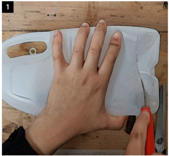
1 Wash the milk bottles and remove all labels and stickers. Pierce into the milk bottle using a box knife.
