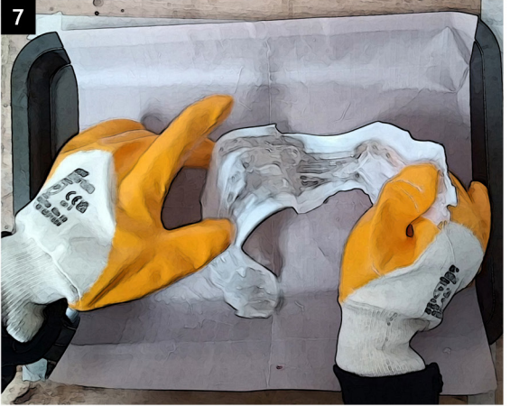
7 Shape the plastic by hand, creating a wave-like shape.
