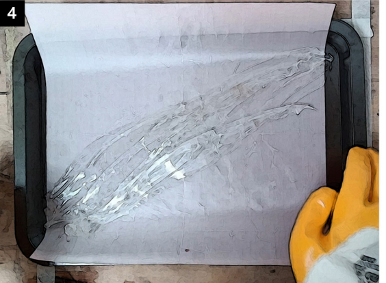
4 Place the baking tray in the oven at the temperature of 180°C for roughly 15 minutes. Melted HDPE looks transparent.
