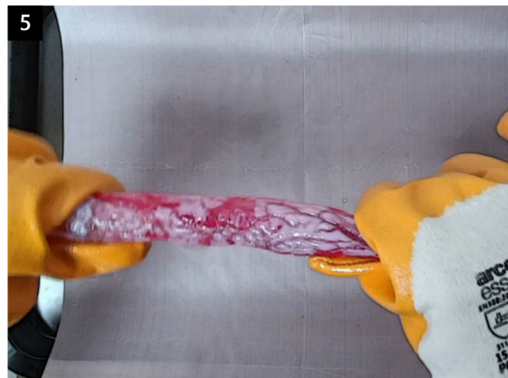
5. Twist the plastic to create a long rolled tube and twist the rolled tube to ensure that the color blends well. Pull the tube to elongate it.
