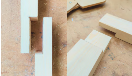
Fig. 88. Half Lap Joint, (2024)
