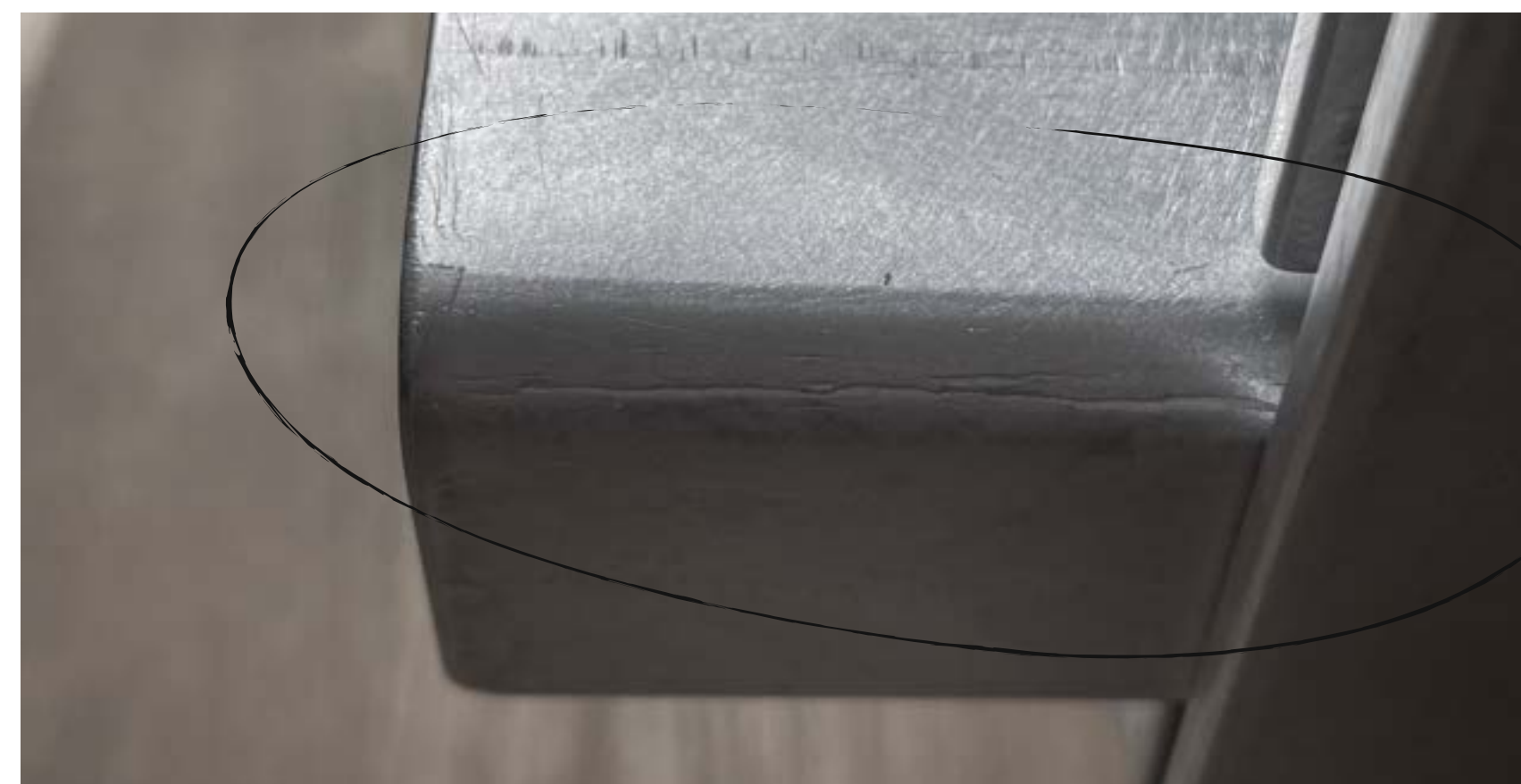
Fig.26. cracked bend part, Linda Suchanová
