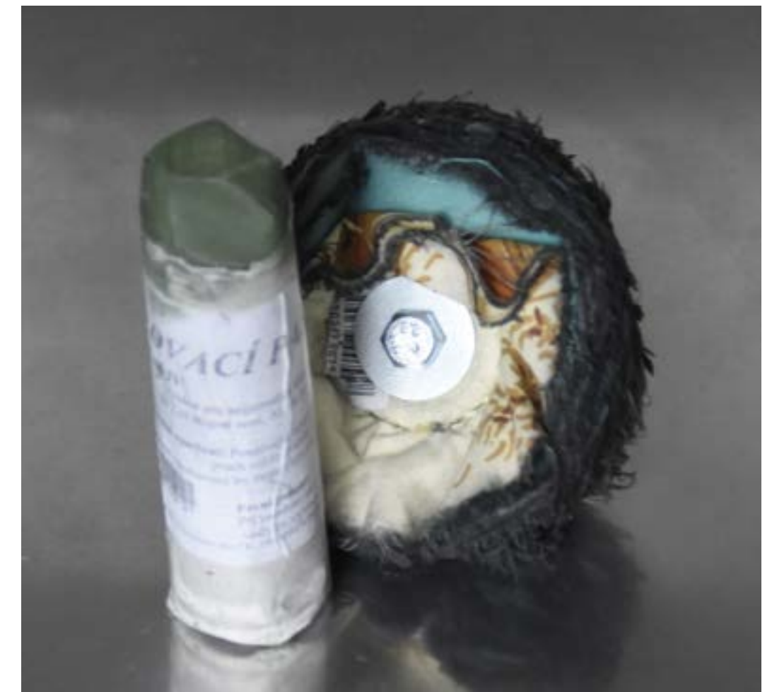
Fig.31. polishing paste 2, fabric polishing wheel, Linda Suchanová
