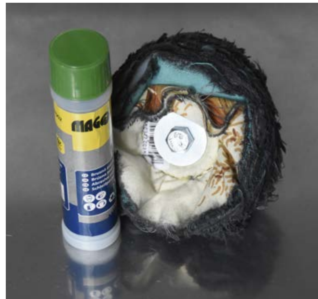
Fig.30. polishing paste 1, fabric polishing wheel, Linda Suchanová
