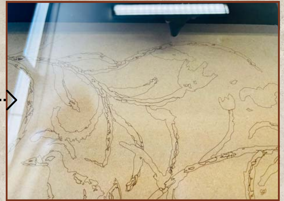
Fig23: Engraved the design onto a MDF board through lazer cutting machine
