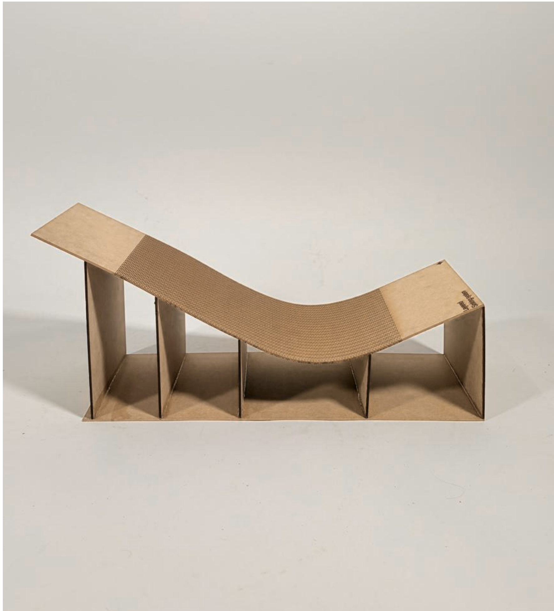
The 1:1 prototype tests how the layered sinking landscape can be physically formed through a flexible surface and variable rib structure. Kerf-cut MDF was used as fabrication medium to explore curvature, support spacing and the relationship between soft and rigid material layers.
